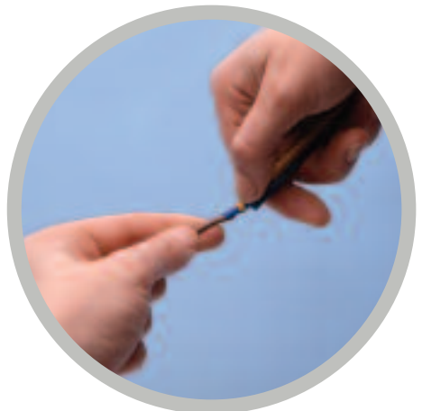
Push marker onto cable
